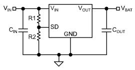
The shutdown pin on the MIC79110 can be used to automatically shutdown the battery charger when the input voltage rises above a safe operating voltage. To keep the part from heating up and entering thermal shutdown, we can connect the shutdown pin to  $V_{\text{IN}}$  using a resistor divider. Use the following equation to setup the maximum  $V_{\text{IN}}$ .
