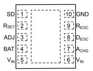
Adjustable Output 10-Pin 3mm × 3mm MLF<sup>®</sup> (ML)
