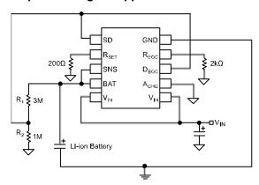
Lithium-lon batteries will begin to lose their charge over time. The MIC79110 can be configured to automatically recharge the battery if the voltage drops below a certain voltage. This minimum voltage is set by a resistor divider at the battery and connected to the SD pin. When the battery voltage falls below the minimum voltage, the SD pin is pulled low to start the normal charging process.
