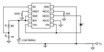
This circuit is similar to the auto top off charger circuit mentioned above except that the  $D_{EOC}$  pin is externally triggered to restart the charging cycle. It still uses the same resistor divider to set the minimum battery voltage before the lithium-ion needs to be recharged.
