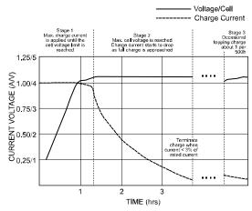
All lithium-ion batteries take approximately 3 hours to charge with the second stage taking twice as long as the first stage. Some chargers claim to be fast chargers by skipping the second stage and just charges the battery until the cell voltage is reached. This only charges the battery to 70% capacity.
